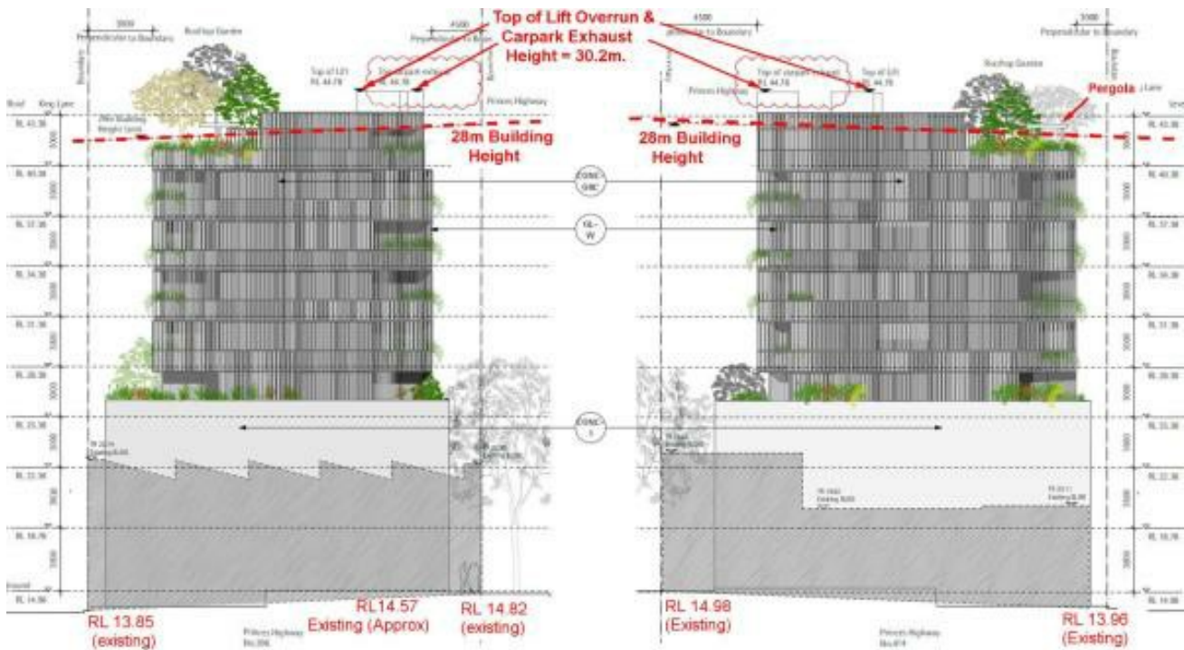
Figure 5 - Building Height exceeding maximum 28m height limit (Princes Highway frontage)
